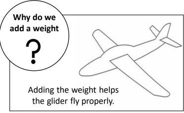
The nose weight is added to help bring the balance point (centre of gravity) of the glider to just in front of the wings. This helps the glider to be stable in the nose-to-tail direction.
